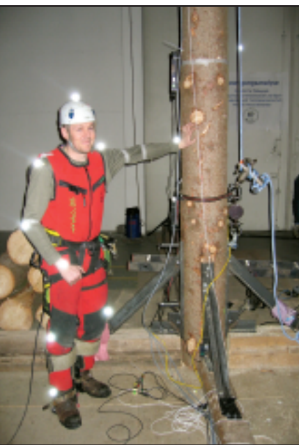
Figure 2. Tracking the motion of the climber. Two strain gauges (Elastometers; red arrows) measure stretch in marginal fibers if the stem bends under load (pulling it to the right in this picture).
